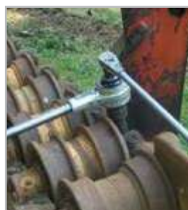
Torque multiplier used on tracks
