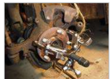
3 Jaw Puller used for removing tyre hub
