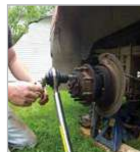
Torque multiplier used for lug nuts
