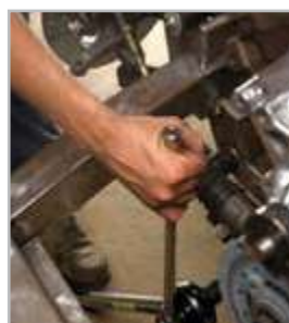
Torque multiplier used in inaccessible areas
